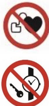
People with other metal or electronic surgical implants are not allowed to work with the OC 0350 and must maintain a safety distance of at least 1 m from the device.
